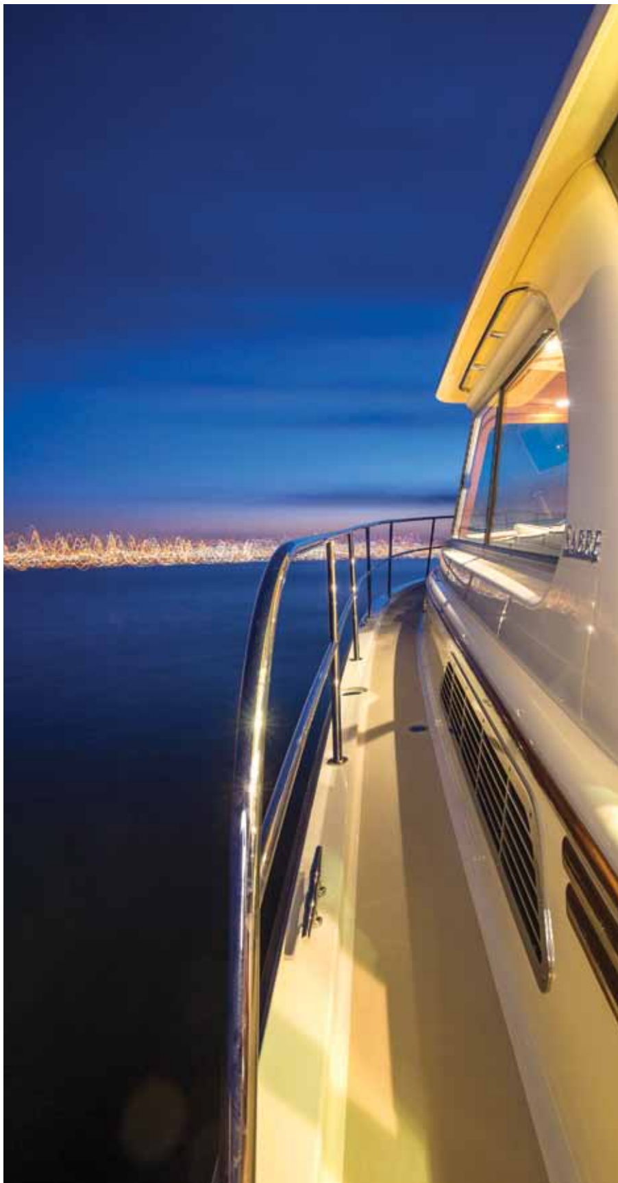
Get a grip for safe passage forward with a good high bowrail and a grabrail on the house.
