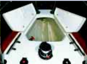
The divided anchor locker with windlass
